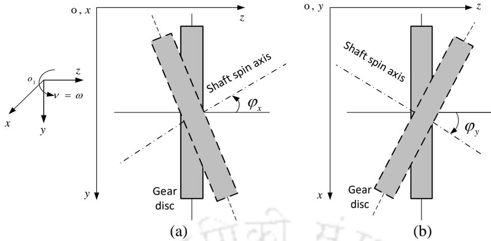
**Figure 2** Coordinate axes and positive conventions for rotational displacements due to gyroscopic effect (a) tilting of shaft axis  $y$ - $z$  plane (b) tilting of shaft axis  $z$ - $x$  plane
