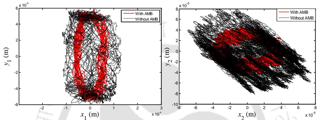
**Figure 5** Comparison of orbit plot after AMB control (a) Input end (a) Output end
