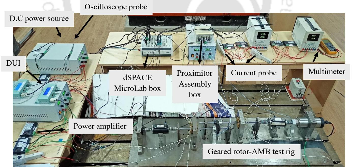
**Figure 4** Control Architecture of Experimental Rig
