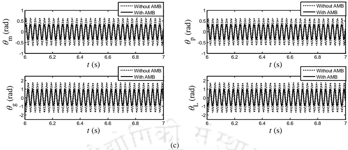
**Figure 3** Time domain response at  $\omega_p = 60\text{Hz}$  ,  $\omega_g = 30\text{Hz}$  ,  $\omega_e = 1500\text{Hz}$  (a) x, y displacement of input shaft (b) x, y displacement of output shaft (c) torsional displacement of motor, pinion, gear, load respectively.
