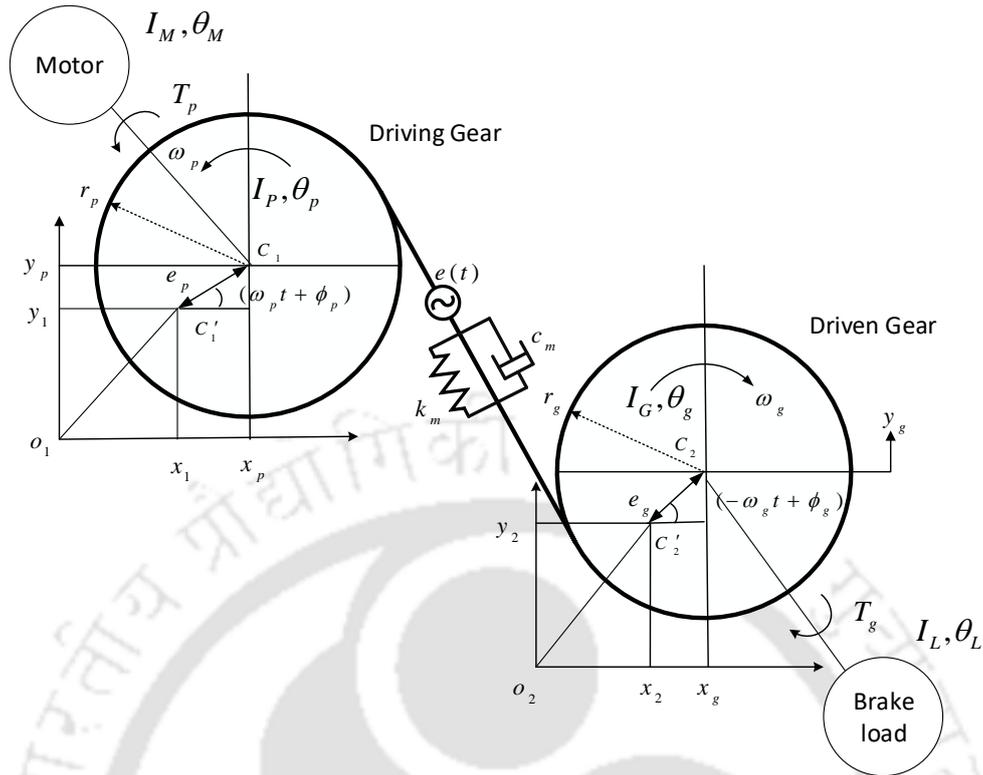
**Figure 1** Gear mesh model with co-ordinate system
