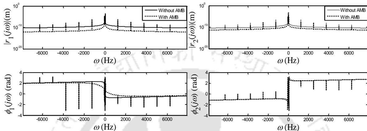
**Figure 6** Full spectrum response generated at  $\omega_p = 60\text{Hz}$  ,  $\omega_g = 30\text{Hz}$  ,  $\omega_e = 1500\text{Hz}$  (a)
