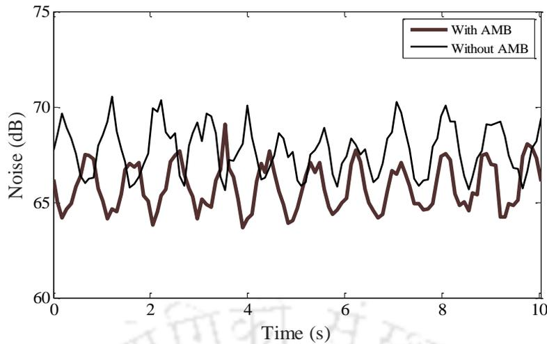
**Figure 7** Comparison of overall reduction in radiated gear noise levels after AMB control.
