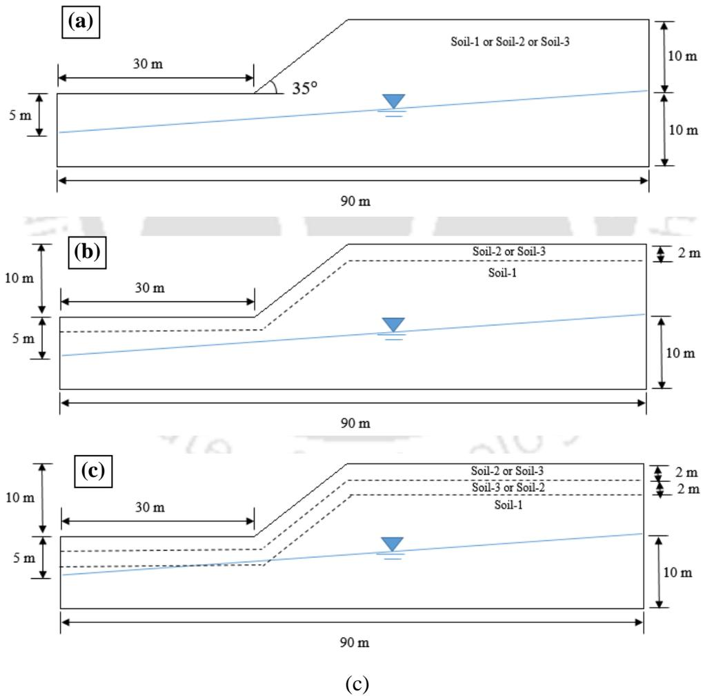
Figure 4 Models used for infiltration analysis: (a) Homogeneous slope (b) Two-layered slope (c) Three-layered slope
