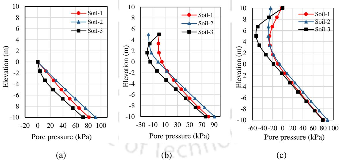
Figure.8 Pore-water pressure profiles for homogeneous slopes with different soils after 24 hours along different sections at: (a) Toe, (b) Mid-slope, and (c) Crest
