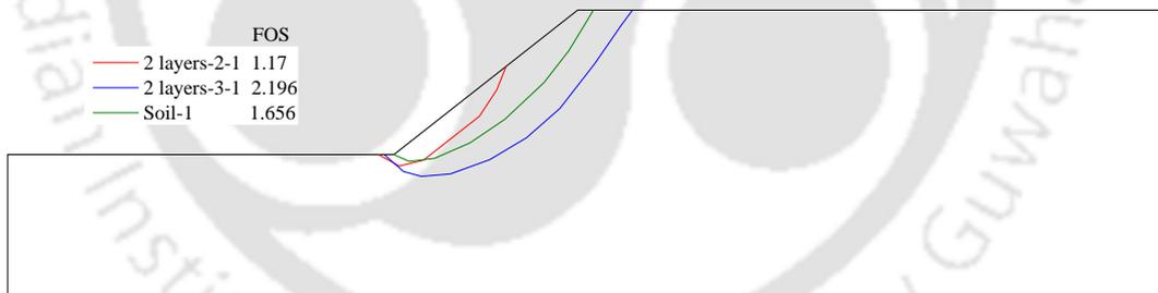
Figure 15 Critical slip surfaces for the non-homogeneous slopes after 24h
