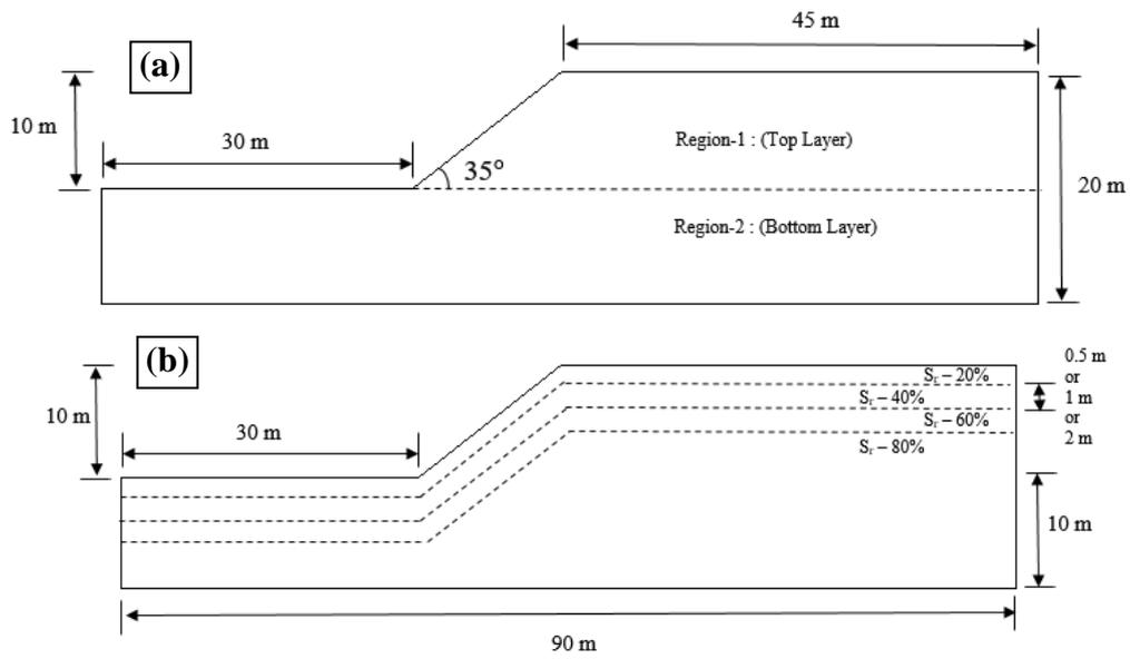
Figure 3 (a) Two-layered non-homogeneous slope model (b) Multi-layered slope model with layers representing different moisture levels increasing with depth
