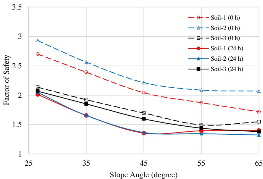
Figure.10 Variation of safety factor with slope angle for the three soils at the initial stage and after 24 h
