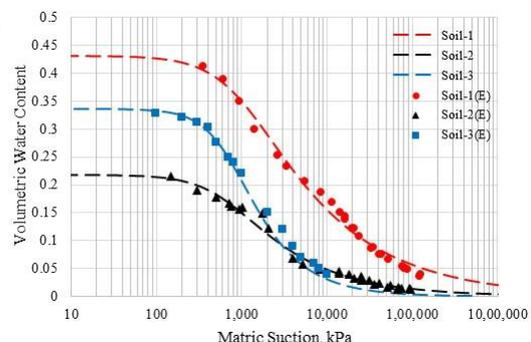
Figure 2 SWCC of the three soils used in the study
