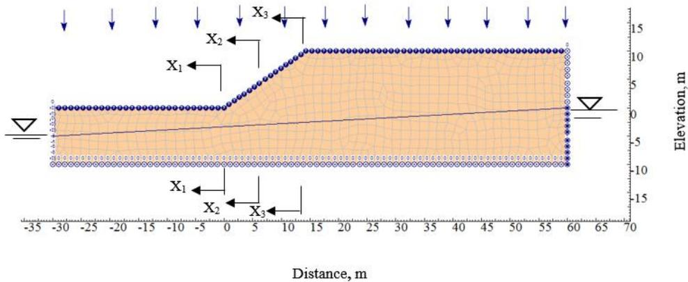
Figure 5 Model of the slope used in study for infiltration analysis
