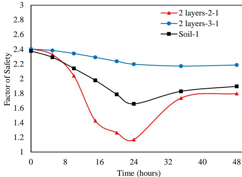
Figure 14 Variation of a factor of safety with time for the non-homogeneous slopes
