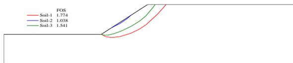
Figure.6 Critical slip surfaces for the homogeneous slopes
