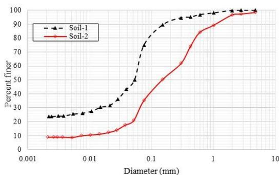
Figure. 1 Particle size distribution curves of the soils used
