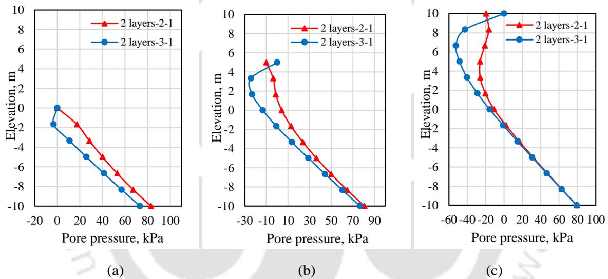
Figure 13 Pore-water pressure profiles for layered non-homogeneous slopes after 24 hours along different sections at: (a) Toe, (b) Mid-slope, and (c) Crest
