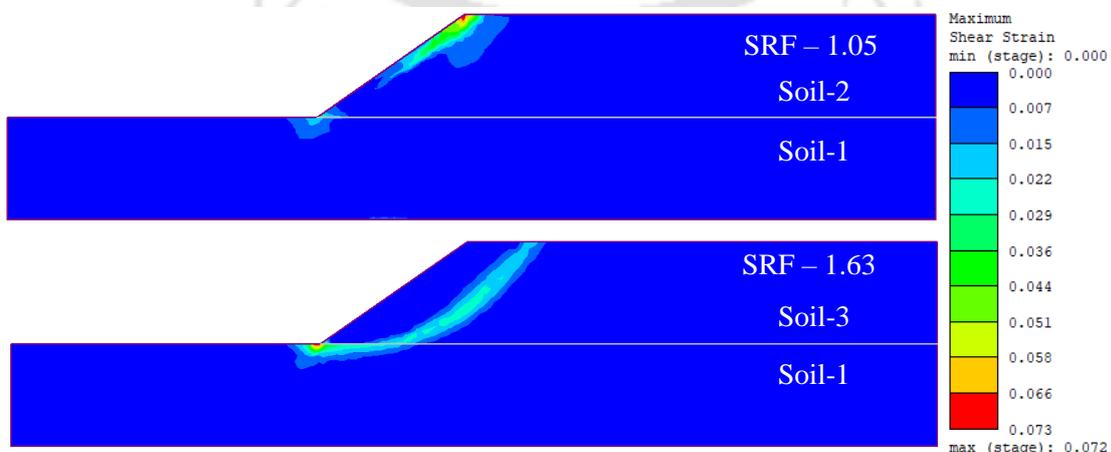
Figure 12 Maximum shear strain contours for the two-layered slope at  $h=0.5D$
