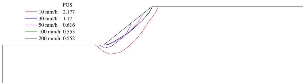
Figure 16 Critical slip surfaces for the two-layered slope after 24 h under different rainfall intensities
