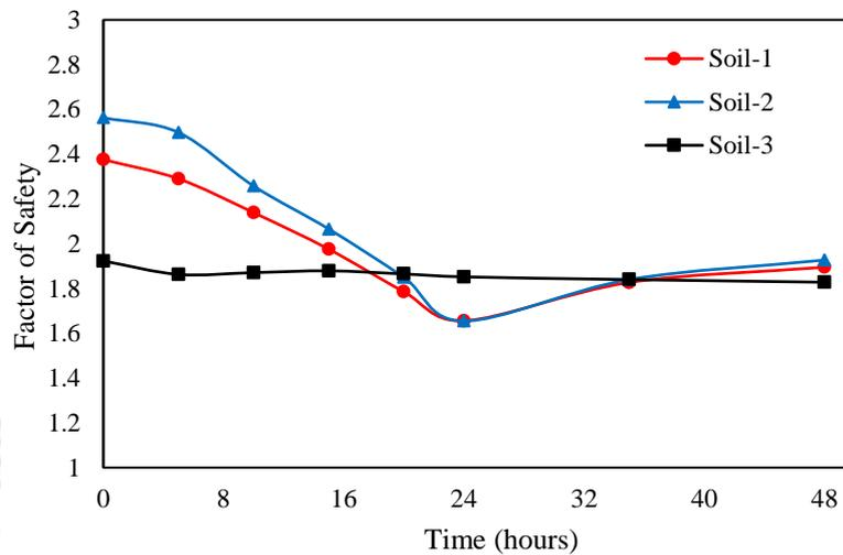
Figure.9 Variation of safety factor with time for the homogeneous slopes
