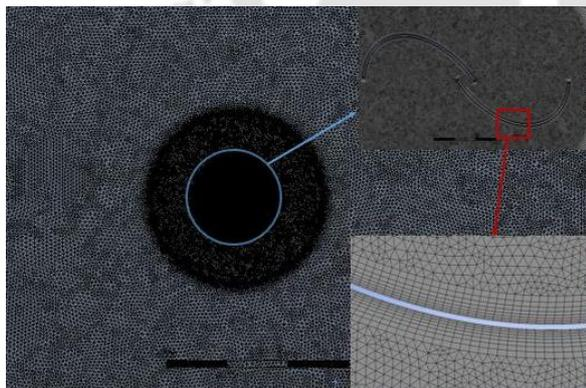
Fig. 3: Mesh generation around the rotor
