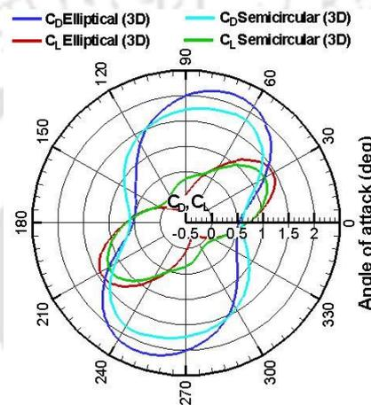
Fig.11: Variation of the 3D  $C_D$  and  $C_L$  for the elliptical and semicircular-bladed rotors at  $TSR = 0.6$ .
