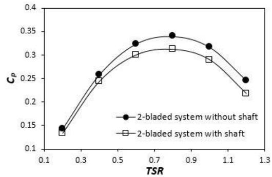
Fig. 8:  $C_P$  vs  $TSR$  for the elliptical-bladed profile without and with shaft
