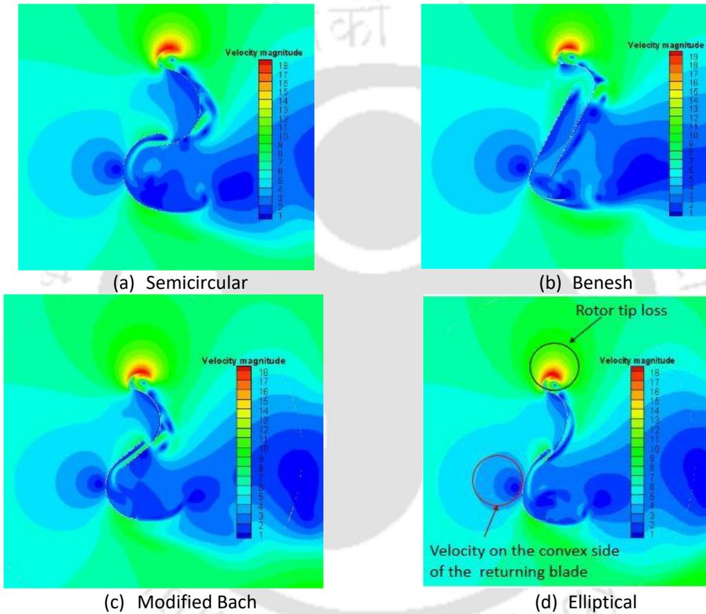
Fig. 6: Velocity magnitude (m/s) of various rotor profile at TSR = 0.80
