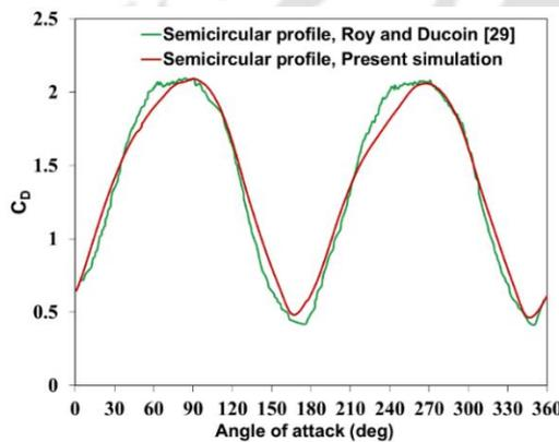
Fig. 9: Validation of present 2D  $C_D$  with the available results.
