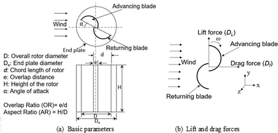
Fig. 1: Illustration of basic parameters and forces of Savonius rotor
