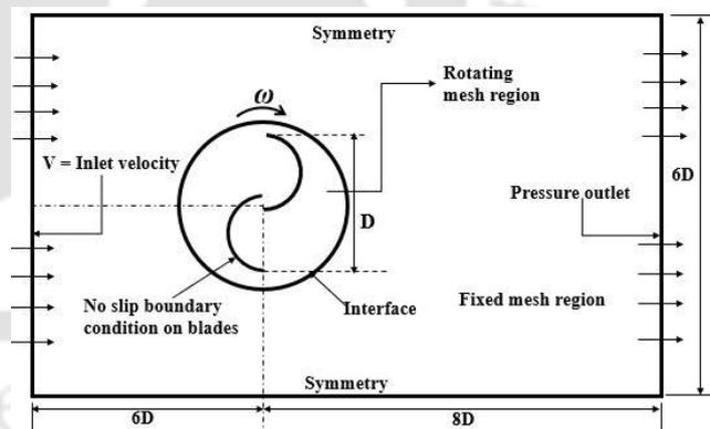
Fig. 4: Boundary Conditions and Computational Domain.
