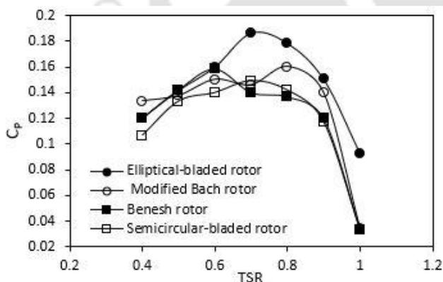
Fig. 14: Performance coefficients obtained from wind tunnel experiments
