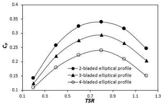
Fig. 7:  $C_P$  vs  $TSR$  for 2-, 3- and 4-bladed elliptical profile
