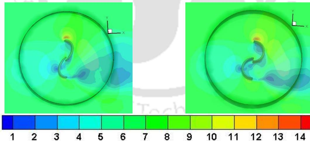
Fig.12: Velocity magnitude (m/s) contours of elliptical and semicircular bladed rotors at  $TSR = 0.6$
