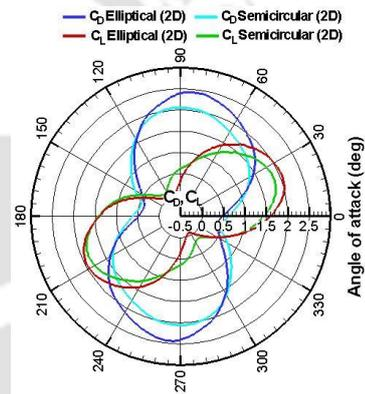
Fig.10: Variation of  $C_D$  and  $C_L$  for the elliptical and semicircular profiles at  $TSR = 0.6$ .
