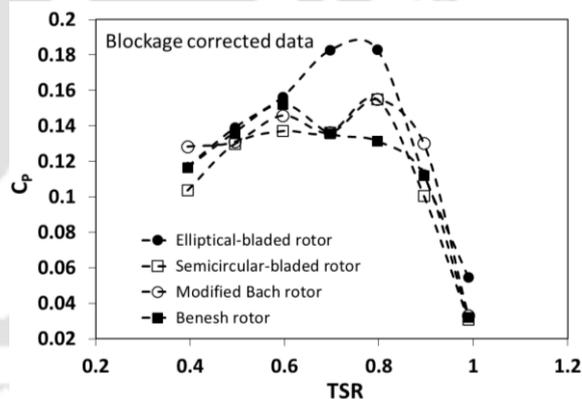
Fig. 15: Blocakge corrected performance coefficient.
