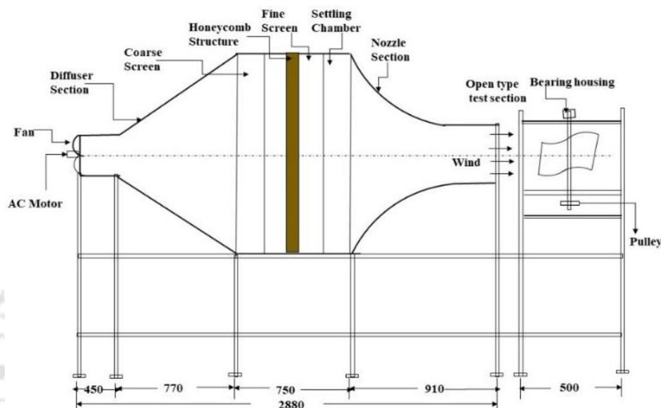
Fig. 13: Schematic diagram of a wind tunnel.
