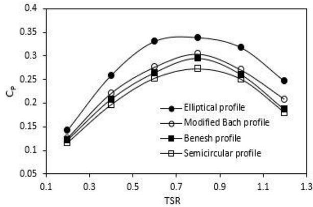
Fig. 5: Performance coefficients obtained from 2D numerical simulation
